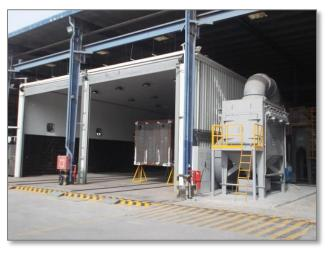
This state of the art blasting booth is fully enclosed and has a full dust extraction system, an under floor grit recovery and recycling system, appropriate firefighting system and an effective waste management system. This gives the Production Team the capability to blast and paint products in the Specialist Services Jebel Ali Centre of Excellence yard.
